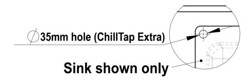
Position the Tap such that it dispenses into the sink bowl with ample clearance for a cup or a carafe. Alternatively, the Tap could be mounted away from the sink using a Zip Font, available as an accessory.
