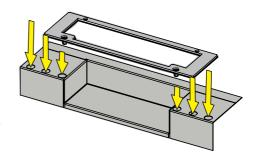
• Fit the Command Centre onto the Mounting Plate.
